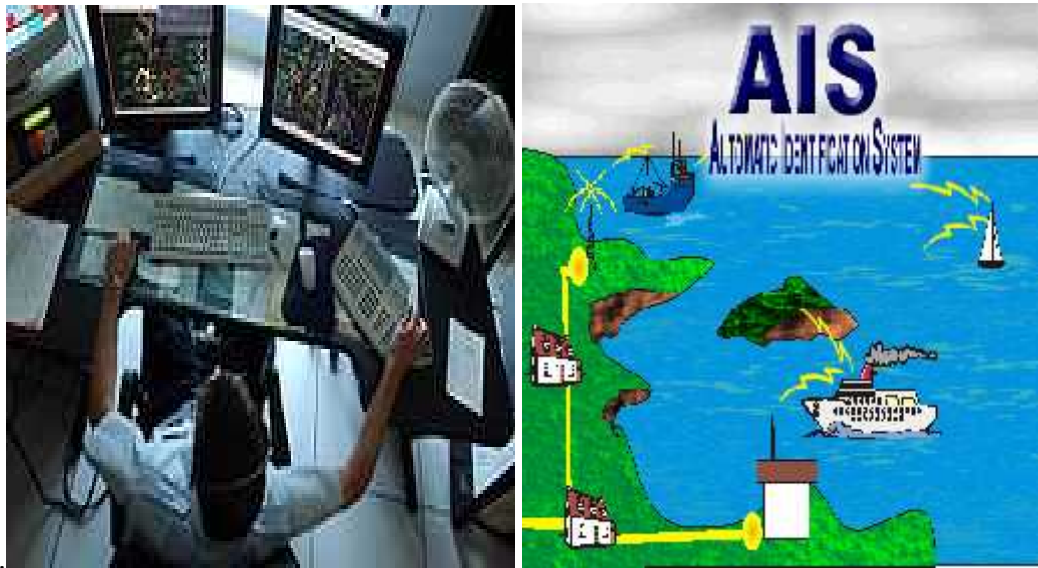
A marine traffic coordinator using AIS and radar to manage vessel traffic
